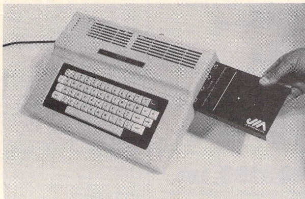
THE J & M SYSTEMS COCO DISK CONTROLLER plugs into the cartridge slot of the Radio Shack Color Computer. It works with either the old or the new models.
